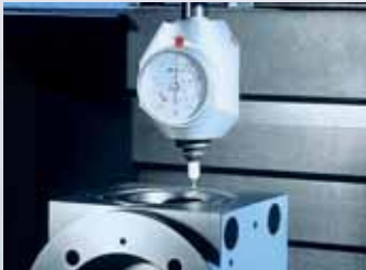
Setting up a part for milling with a 3D sensor
