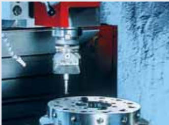
Machining a die-opener disc with the boring tool
